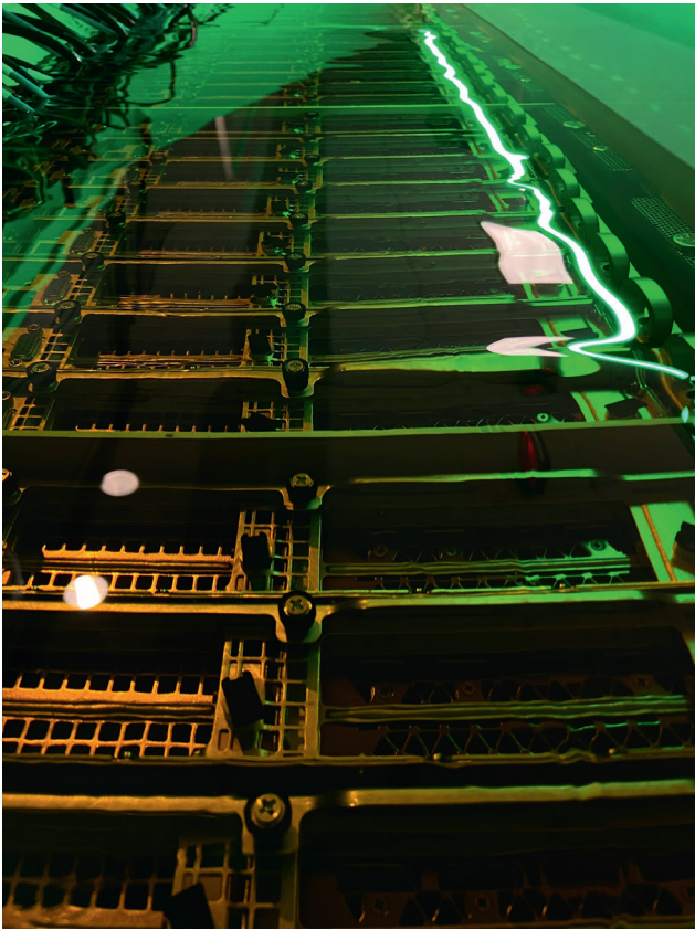
Figure 2 High-density GPU servers submerged in oil.
