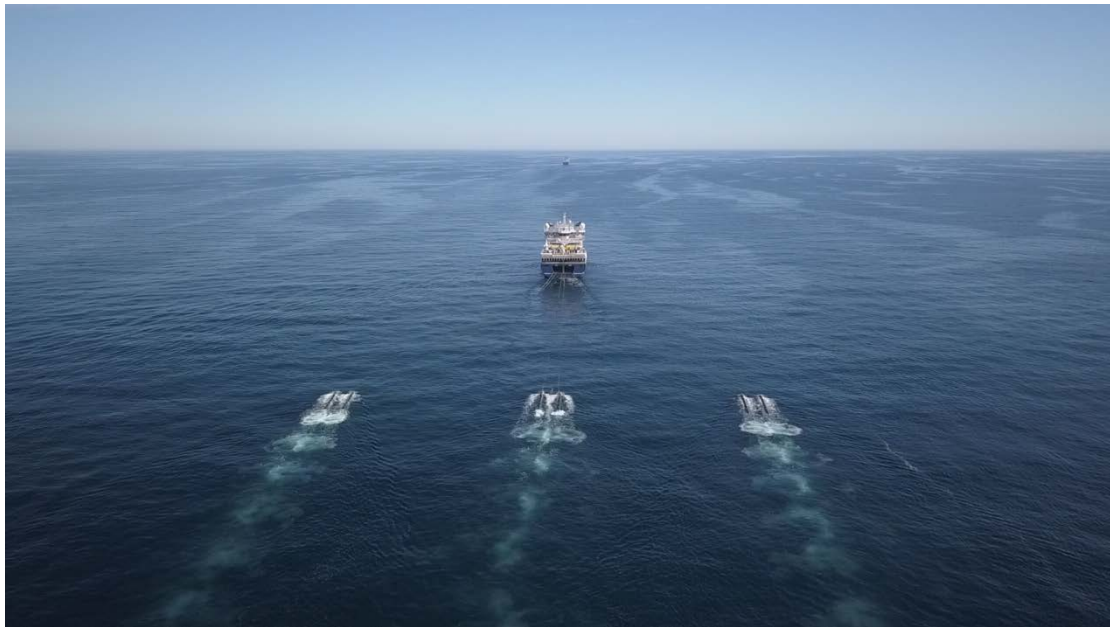
During the TopSeis survey in the Barents Sea the CGG Geo Caspian (seen in the foreground) positions the seismic sources directly over the streamer spread towed by the CGG Geo Coral (background) (image courtesy of CGG).
