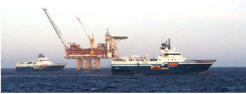
Figure 9 Geo Coral and Geo Caribbean undershooting the Gudrun platform (image courtesy of Equinor).
