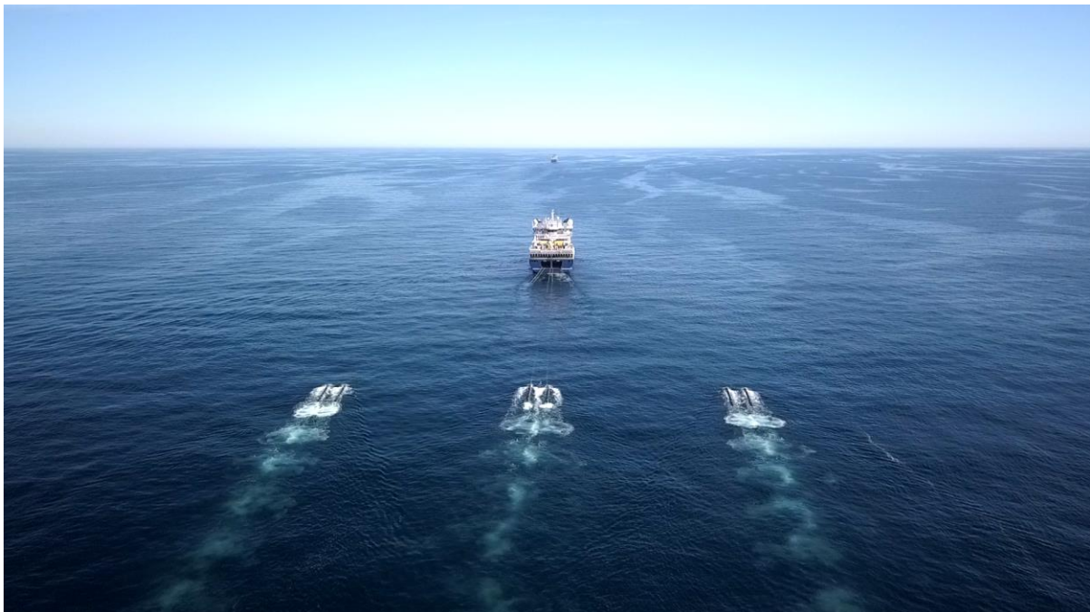
Figure 1: Source vessel shooting over the seismic cables in the Barents Sea. (Photo courtesy, CGG). The streamer vessel can be seen in front of the source vessel, close to the horizon. She is towing 14 streamers of 7km length. The source vessel is towing a new compact designed triple-wide-tow source with only 8.33m shot point interval.
