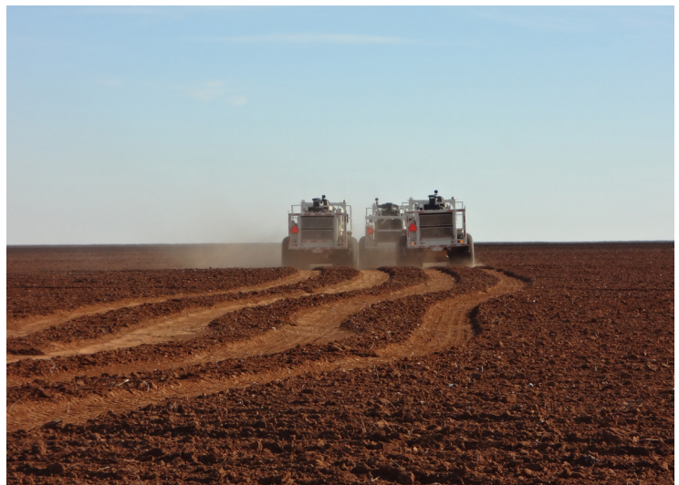
Figure 6. Vibrator group acquiring in a ploughed field.
