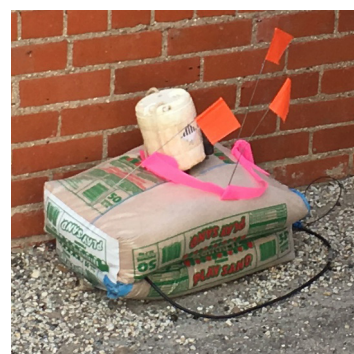
Figure 8. Urban receiver: node unit with geophone spike stuck into sandbag.
